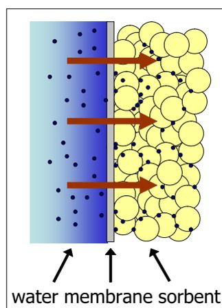
**Figure 2.1** General passive sampling principle: substances (black dots) traverse through a diffusion barrier into the passive sampling device where they are entrapped by a receiving phase.
