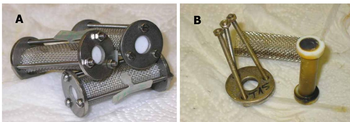
**Figure 5.1** Exemplary photographs of Toximeters taken out of borehole 3 (A) and borehole 2 (B) after 3 months of exposure.
