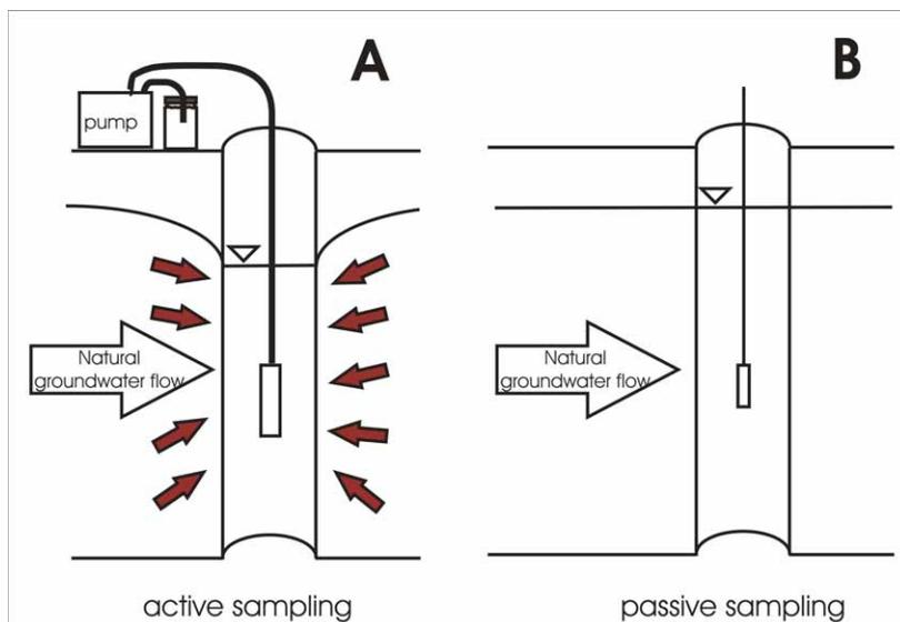
**Figure 1.1** Comparison of active (A) and passive (B) groundwater sampling.
