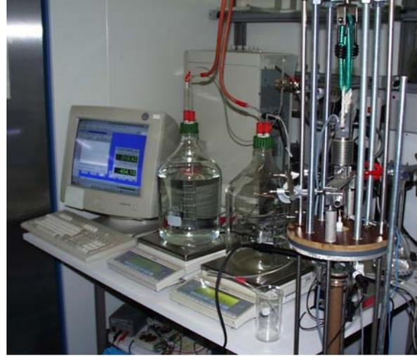
**FIGURE 14:** Sand-filled, dynamically compressed symmetrical column (left), computer based data recording in the outlet of the column (right).
