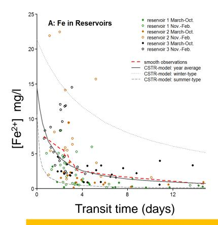
Fast binding of PO<sub>4</sub> in presence of Fe<sup>2+</sup>: No time for dissolved transport
