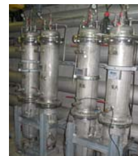
Fig. 2: Groundwater from Zeitz is pumped over these columns, allowing the attachment and growth of microorganisms at the gravels.
